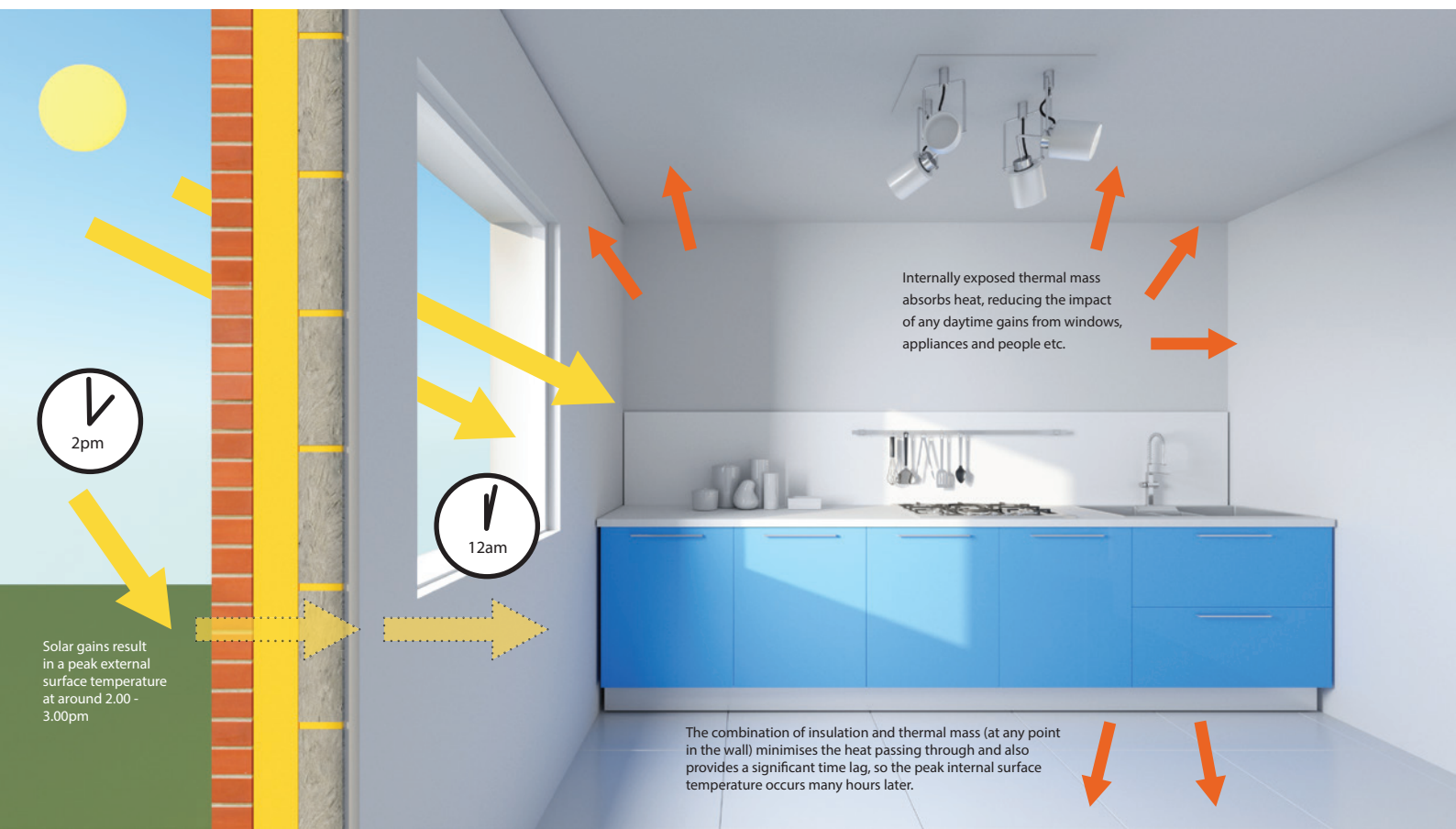
Figure 10: On hot days, internally exposed thermal mass helps counter the impact of heat gains from windows and internal sources. At the same time, the overall mass and insulation provided by the external walls reduces and slows heat gains passing through them, helping ensure that any effect they may have on the internal environment does not occur until late evening/night when the risk of overheating has moderated.
